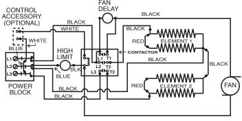
CAUTION: Field wiring must be #10 AWG. min. rated 90°C. min.
