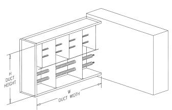
Figure 70. Flanged Duct Heater
