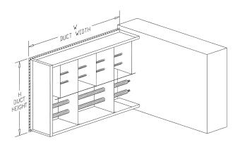
Figure 69. Slip-in Duct Heater
