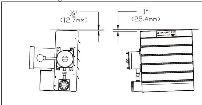
2. To ensure proper heating of floor surfaces, observe the following recommended maximum mounting heights (to bottom of heater):
