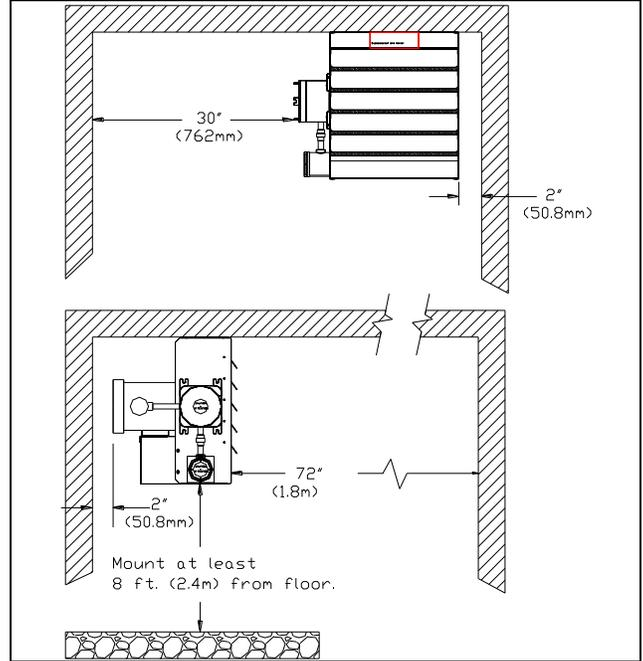
5. The heater may be suspended from overhead beams or mounted to a side wall or a 4" pipe using one of the approved mounting kits. Use of non-approved mounting kits voids all warranties, expressed or implied.
