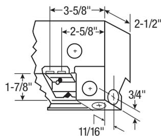
All knockouts are 7/8" diameter for 1/2" conduit
