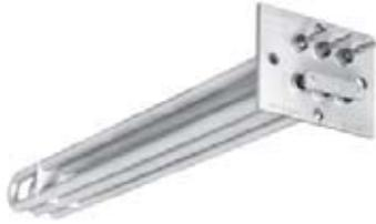
**Large Diameter Elements** provide extra electrical insulation for superior dielectric strength. Because elements are .475" diameter, they are suitable for line voltages up to 600 volts. In addition, element insulation is compacted to insure uniform heat transfer from coil to sheath and all bends are repressed to insure insulation integrity in this critical area.
