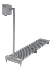
**Sludge Leg Spacers** - To prevent burnouts from spot overheating and to keep elements out of sludge that normally collects in the bottom of the tank. Standard legs are 1-1/2" high; lengths up to 4" are available at no extra charge.
